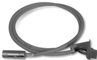
For motors with or without holding brakes, shielded, preassembled on both sides, drag chain suitable and highly flexible (5 bend cycles) cables with round plugs on the motor side and module connectors.
